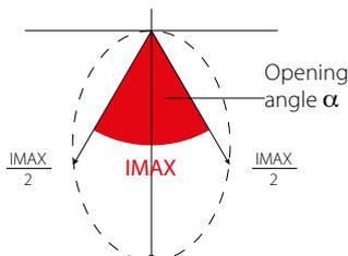
**IMAX** = maximum luminous intensity, i.e. the maximum intensity of the emitted light beam.
